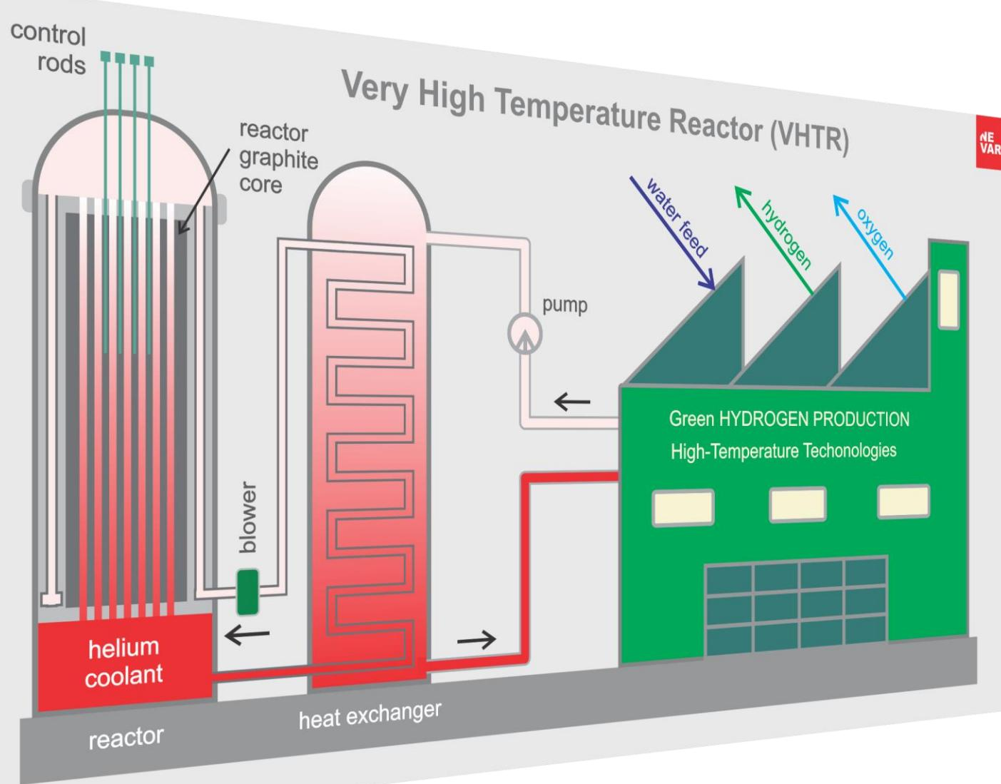
The figure shows a schematic representation of the **VHTR** (Very High Temperature Reactor), together with the hydrogen production plant connected to it, which is based on the previously mentioned high-temperature technologies—**HTWE** and **TcWSC**. Such a reactor produces heat at temperatures of up to 1000 °C and enables the cogeneration of electricity and hydrogen.
