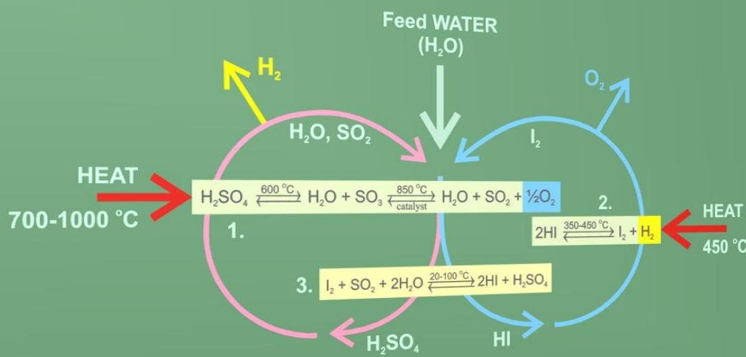
Several different thermochemical concepts for hydrogen production from water have been explored in recent decades, but the most extensively studied is the **SULFUR-IODINE (SI)** cycle. This cycle is considered the most suitable option because it offers the highest efficiency among the proposed methods and operates at temperatures below 1000 °C. Its schematic diagram is shown in the figure.
