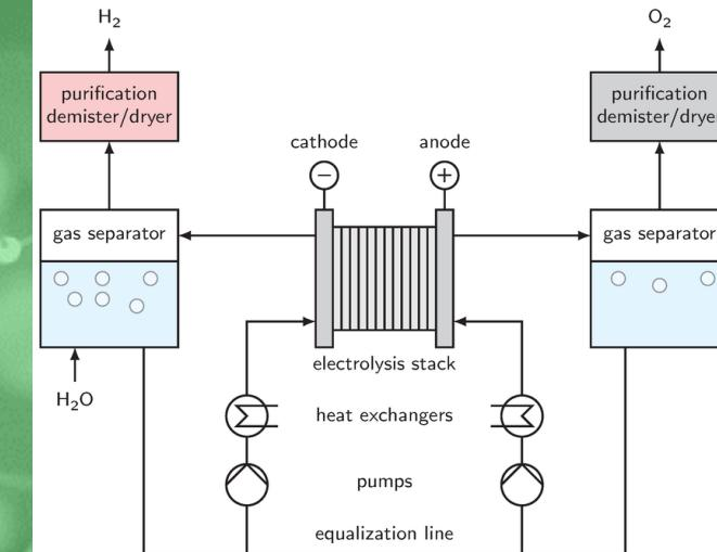
A schematic flow-diagram of an industrial alkaline water electrolyzer.
