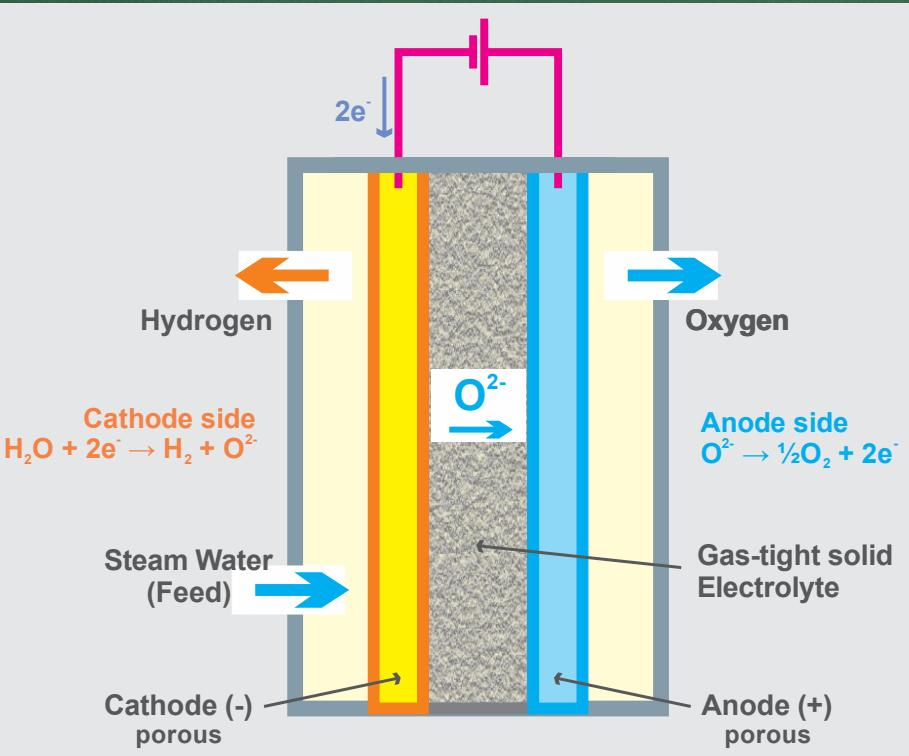
**The principle of HTWE is as follows:** At high temperature and with the help of an electric current, the feed water vapor is decomposed on the cathode side into  $H_2$  and oxide ions ( $O^{2-}$ ). The hydrogen leaves the system as a gas, while the oxide ions migrate through the electrolyte (see figure). They are neutralized on the anode side and released as gaseous oxygen.
